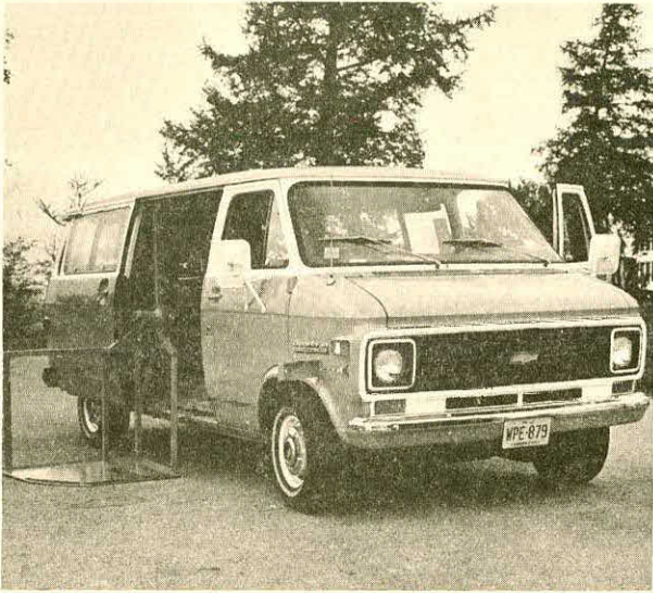
Fig. 7 Chevrolet Sportsvan, equipped with side-loading wheelchair lift (Helper Industries, Ft. Lauderdale, Florida)
