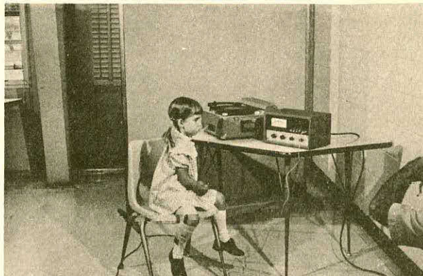
When knee movement stops, Synaptor's warning buzzer sounds before cutting off electricity to the record player.
