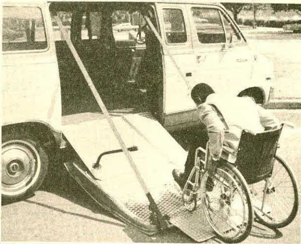
Fig. 8 Dodge Sportsman van, including integral wheelchair entry-exit system (Royce International, Englewood, Colorado)
