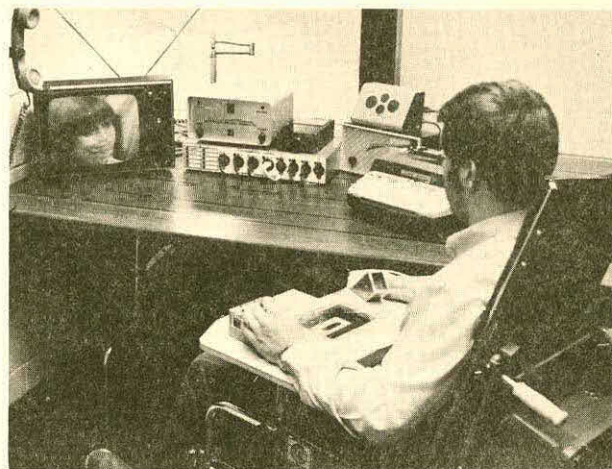
Fig. 7- DU-IT system operating environmental control unit, telephone dialer, TV, intercom and lamp through remote control link.
