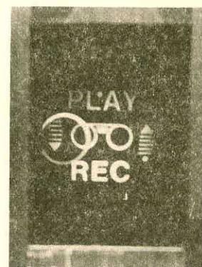
Fig. 4- Tape recorder selection projected on display screen. Circle shows that 'fast backward' function has been activated.
